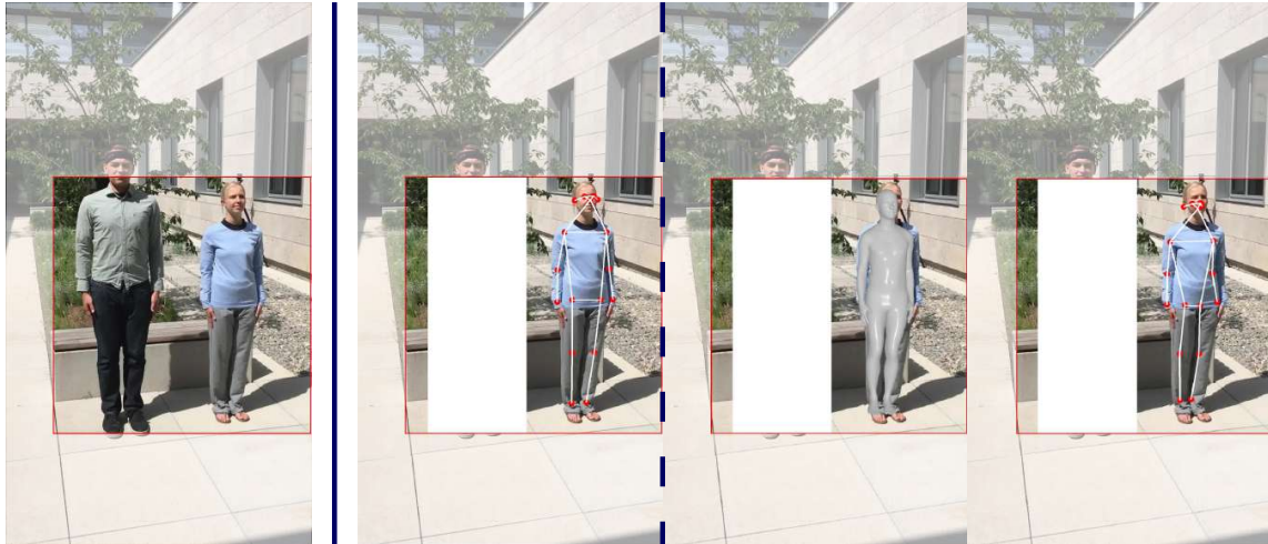
Figure 4.4: Output of second-level processing nodes for an input patch of the same frame as in Figure 4.2. From left to right: input patch derived by resizing and squaring the female’s tight bounding box, estimated 2D pose keypoints in COCO 17 format, projected SMPL mesh generated by the estimated parameters, and its corresponding 2D keypoints. Note that small errors in the resizing of the bounding box that resulted in it being non-square, were propagated to the projection of SMPL mesh and joints. This figure is best seen in zoom.
