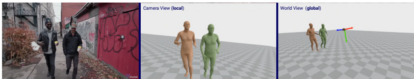
Figure 12: Input, camera-local, and global SMPL mesh placement [7].
