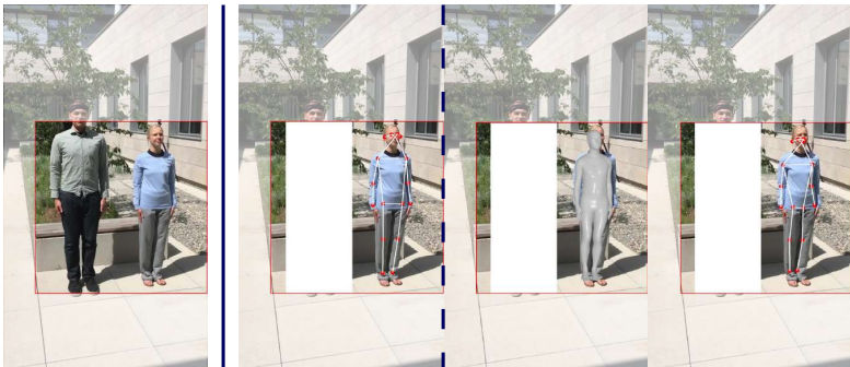
Figure 9: Output of patch-level processing nodes. From left to right: female patch (squarified), estimated 2D pose COCO17 keypoints, projected SMPL mesh and joints. Subject isolation is performed for the male subject.
